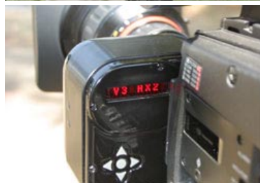
AX2 Parallax Scanning Adapter uses optical scanning techniques to inject 3D-like impressions of depth on standard film or video.
