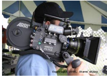
ARRIFLEX 416 S16 film camera, a smaller, lighter 16mm film camera.
